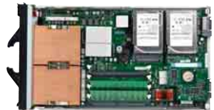
The 2-way HS20 Blade includes models that support Intel Extended Memory 64 Technology, supporting transition to 64-bit applications.
